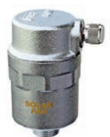
Fig.1 If there is no air in the circuit, water inside the air vent valve keeps the float in such a position as to close the shutter.
