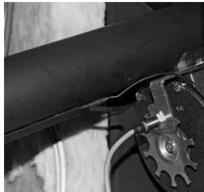
Fig. 21 Inserting sensor and sensor guard into holder on auger tube
