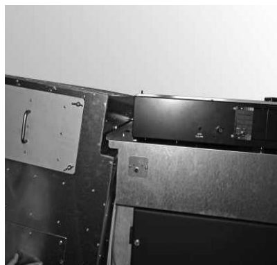
Fig. 24 Fitting the integral fuel hopper
