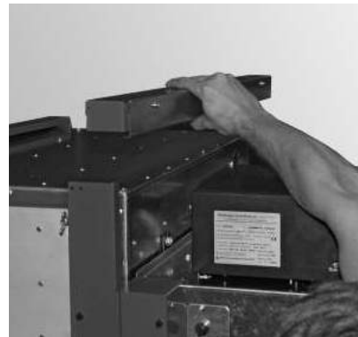
Fig. 52 Mounting hopper cladding at top right
