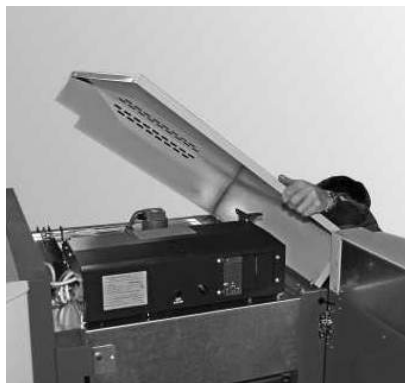
Fig. 79 Fitting the cladding cover
