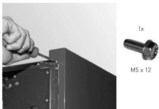
Fig. 50 Securing left side panel to hopper at top rear with 1 TT screw
