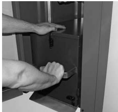
Fig. 73 Pressing the container slightly to the right and sliding the handle all the way in
