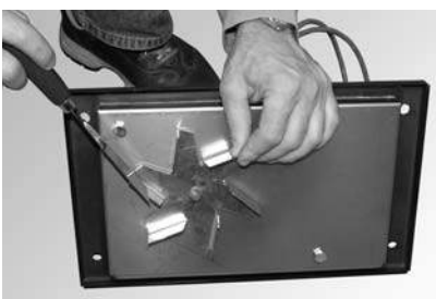
Fig. 132 Cleaning the blower wheel
