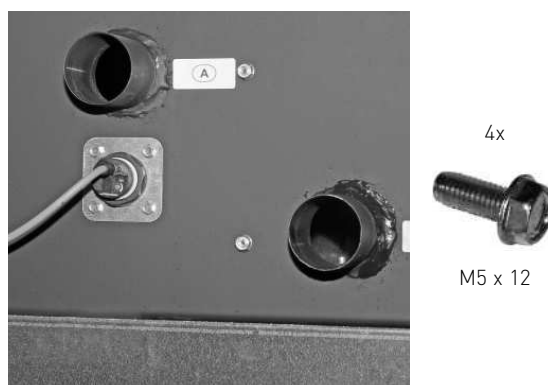
Fig. 33 Mounting „full“ fill level switch to top rear of hopper with 4 TT screws
