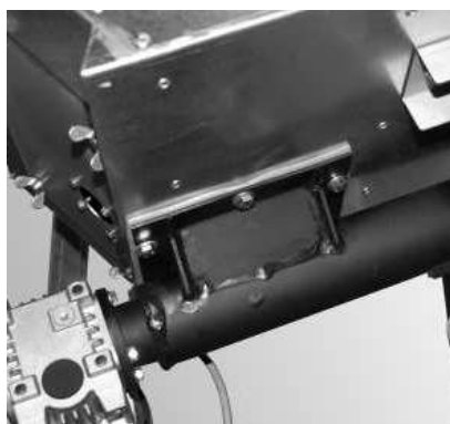
Fig. 29 Fitting auger with 6 U-washers and 6 hexagon screws
