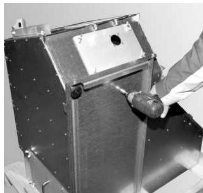
Fig. 10 Remove crate and unscrewing floor plate of integral fuel hopper
