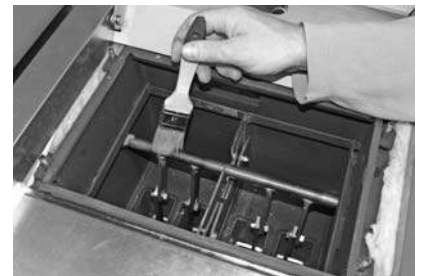
Fig. 131 Cleaning the coating surfaces
