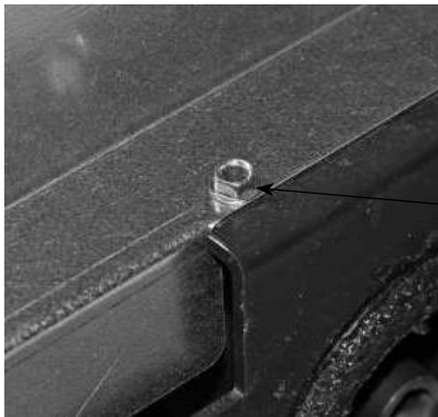
Fig. 47 Securing anti-contact protection plate with TT screw
