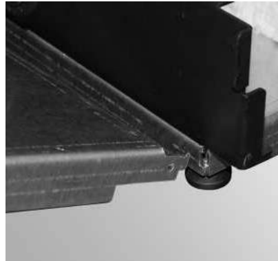
Fig. 13 Attaching the floor plate
