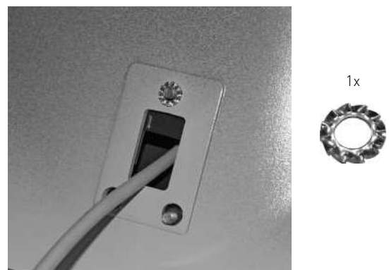
Fig. 62 Fit saw tooth ring under one nut – earthing
