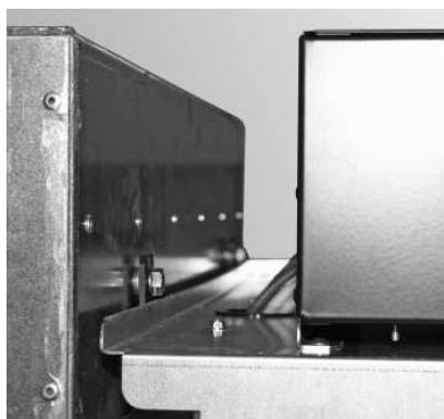
Fig. 25 Tightening 2 TT screws at top
