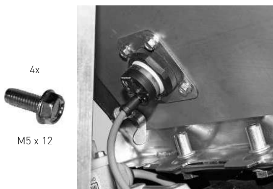
Fig. 32 Mounting „empty“ fill level switch on bottom left of hopper with 4 TT screws
