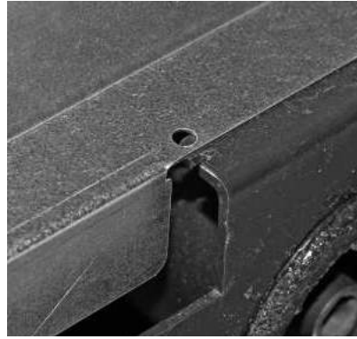
Fig. 46 Sliding anti-contact protection plate into guide slot
