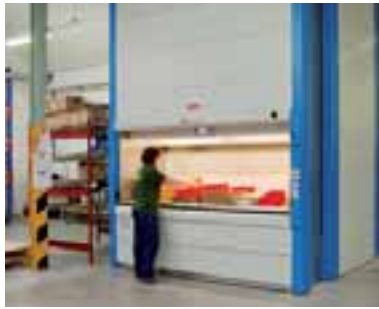
Kardex: automated high-capacity storage system.
