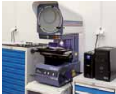
Profile projector at the Quality management laboratory.
