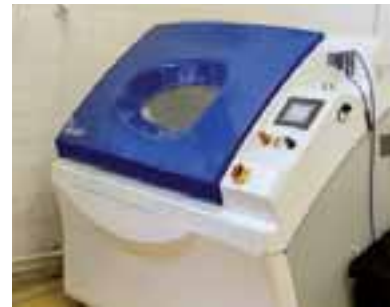
Corrosion chamber to simulate extreme conditions for material testing.
